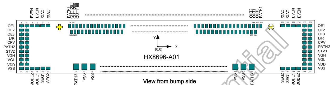
Chip size: 23650 $\mu\text{m}$  x 670 $\mu\text{m}$  (scribe line included)
