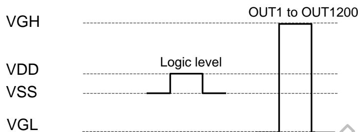
The logic levels of CPV, L/R, OE1, OE2, OE3, /XAO, MODE1, MODE2, SEG1, SEG2, EVEN, STV1 and STV2 have to swing between VDD for "H" and VSS for "L". PATH2 has ESD protection diodes connected to VDD and to VSS, the signal on PATH2 should also swing between VDD and VSS.
