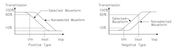
**Vth:** The voltage Vop which the transmission rate of segment is 90%(positive) or 10%(negative) of saturated value on conditions of the selected waveform. (non-selected waveform is opposition)
