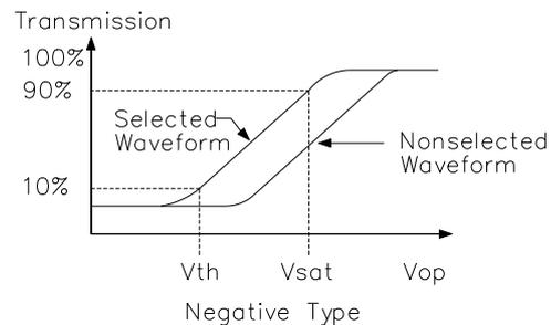
**Vth:** The voltage Vop which the transmission rate of segment is 90%(positive) or 10%(negative) of saturated value on conditions of the selected waveform.(non-selected waveform is opposition)
